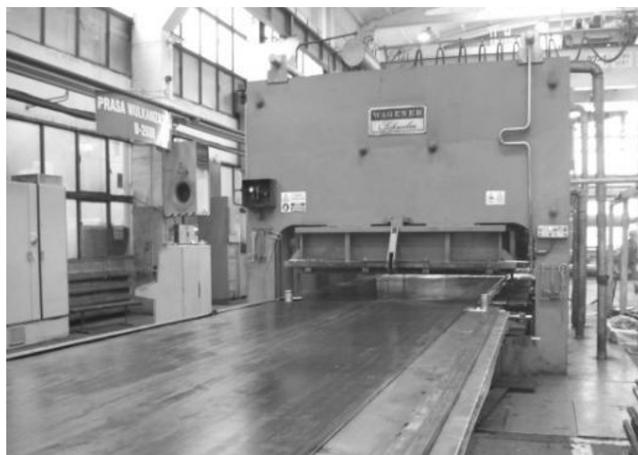
Fig. 7.7. Vulcanization of the conveyor belt in the Wagener heating press Source: own interpretation
