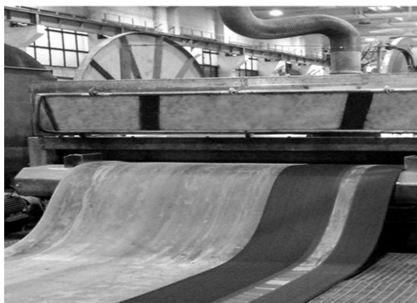
Fig. 7.4. The conveyor belt milling process at the head milling machine Source: Own interpretation
