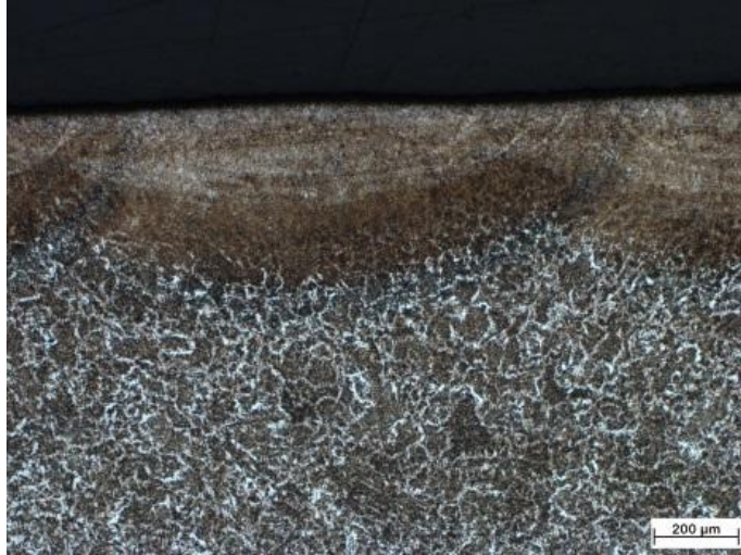
Fig. 12.6. Microstructure in the middle of the laser surface treated weld joint Source: own research
