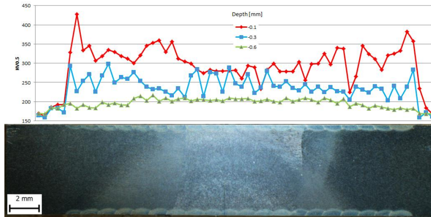
Fig. 12.4. Microhardness profile of the weld surface layer treated by laser Source: own research
