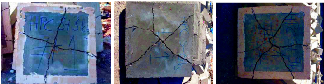
Fig. 4. Crack patterns for High Performance Concrete (HPC)
