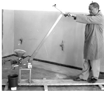
Fig. 2. Operating ram press
