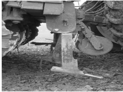
Figure 2. View of the subsoil implements on a chicory lifter.
