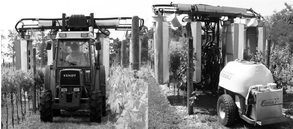
Figure 1. The prototype tunnel sprayer during application in the vineyard.
