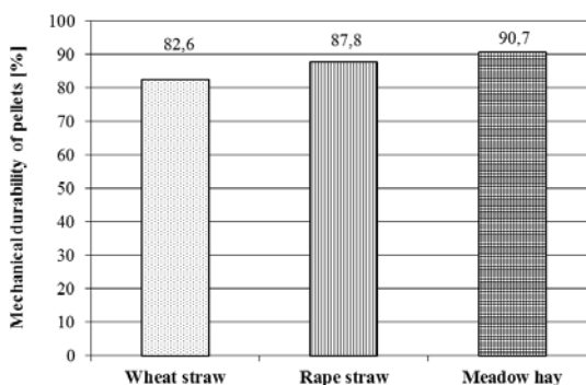
Figure 1. Mechanical durability of pellets produced from plant raw materials
