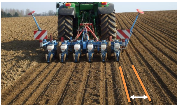
Figure 2. View of the back side of the tractor with the seed drill and the spacing measurement
