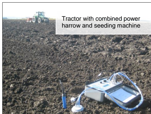
Figure 2. Field measurement (UGT ® ) of soil moisture content (TDR-moisture probe), water tension (tensiometer) and PL-300 measurement chamber for homogenous flow according to DARCY with integrated pressure probe.
