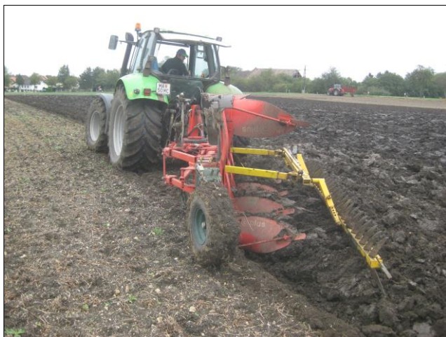
Figure 1. 4 furrow reversible mouldboard plough (Vogel&Noot ® ; 4x45 cm) with mounted furrow slice cracker (Kerner ® )
