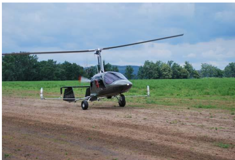
Fig.4. Autogyro equipped with Trichogramma application system
