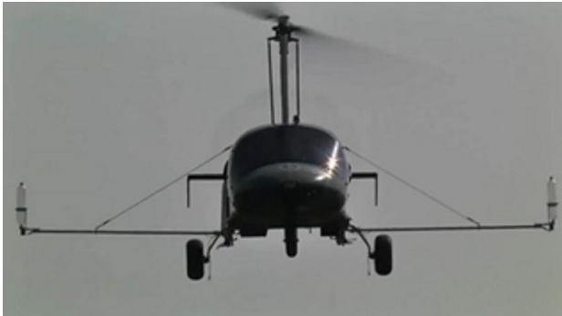
Fig. 1. ZEN1 autogyro with dispensers for biological protection of corn.
