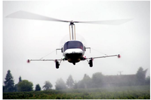
Fig. 2. ZEN1 autogyro for ULV spraying.
