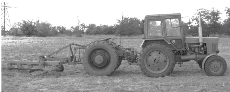
Fig. 1. Ploughing unit on the basis of MPU-80.
