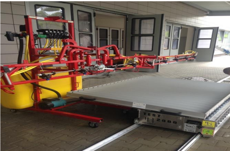
Figure 1. Sprayer test 2000 patternator and the laboratory sprayer boom used in the test
