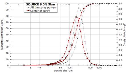
Figure 2. Distribution of droplet size produced by spray
