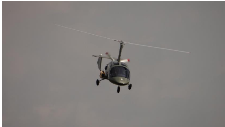
Fig. 1. Gyrocopter equipped with hyperspectral scanners (photo P. Tuross)
