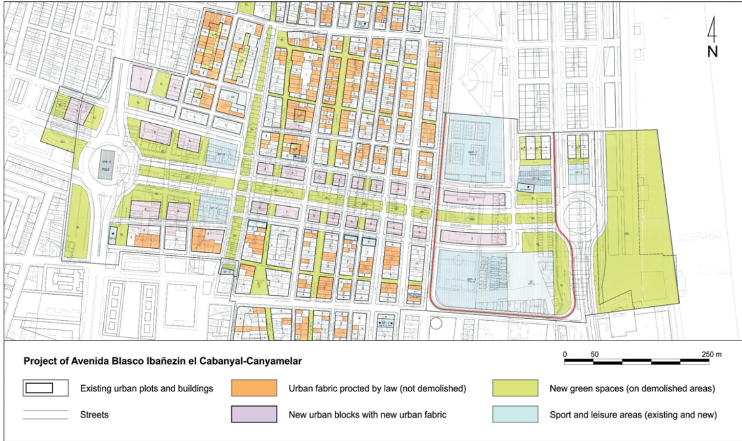
Figure 3. Morphological transformations planned in the central part of el Cabanyal-Canyamelar due to the construction of Avenida Blasco Ibañez and the implementation of the Cabanyal 2010 regeneration plan
