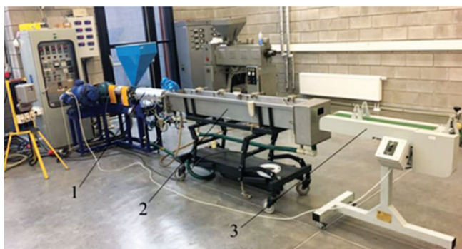
Fig. 1. Technological line of extrusion: 1 – single screw extruder W-25, 2 – cooling bath, 3 – pull-out assembly
