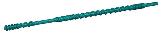
Fig.2 Discrete model of the screw
