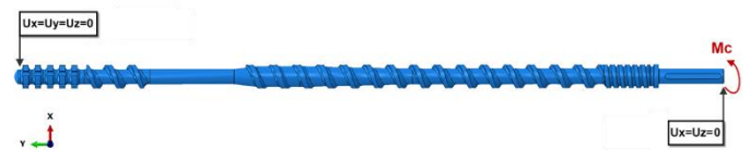
Fig. 3. Definition of the boundary conditions of the screw
