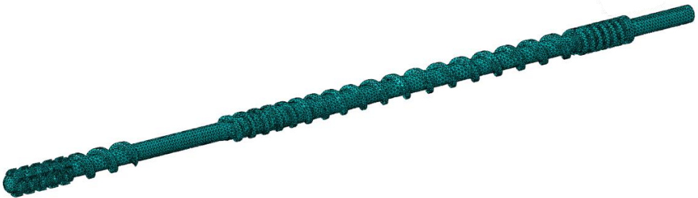
Fig. 26. Discrete model of the special screw – variant 3
