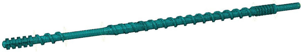
Fig. 24. Discrete model of the special screw – variant 1
