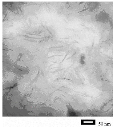
Fig. 16. TEM micrograph of PA/6% Cloisite 30B
