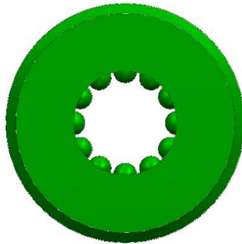
Fig. 39. Cross-section of the rotational barrel segment with the hole with semicircular pins situated alternately in 12 rows
