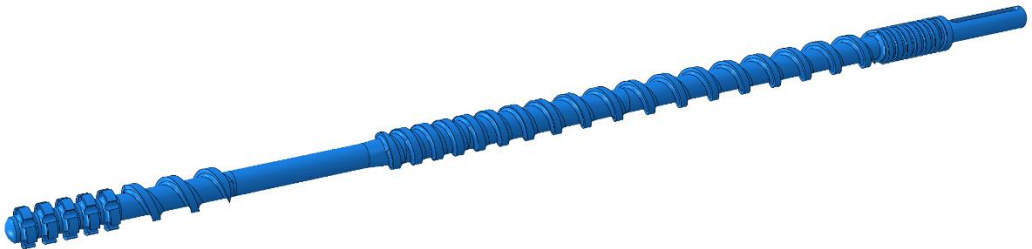
Fig. 20. A special screw model with increasing diameter and decreasing pitch before RBS – variant 2 (concept no 4 – Fig. 9)
