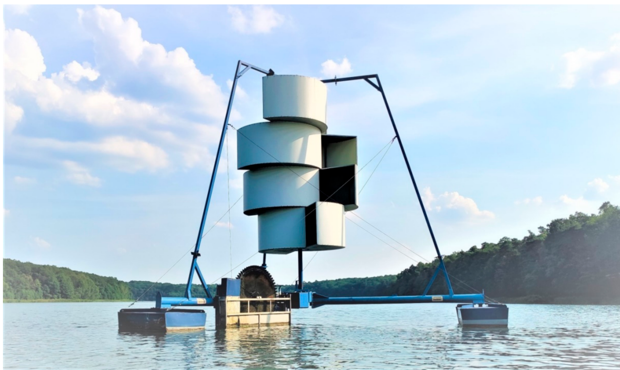
Figure 1. Wind-driven pulverizing aerator—Góreckie Lake.
