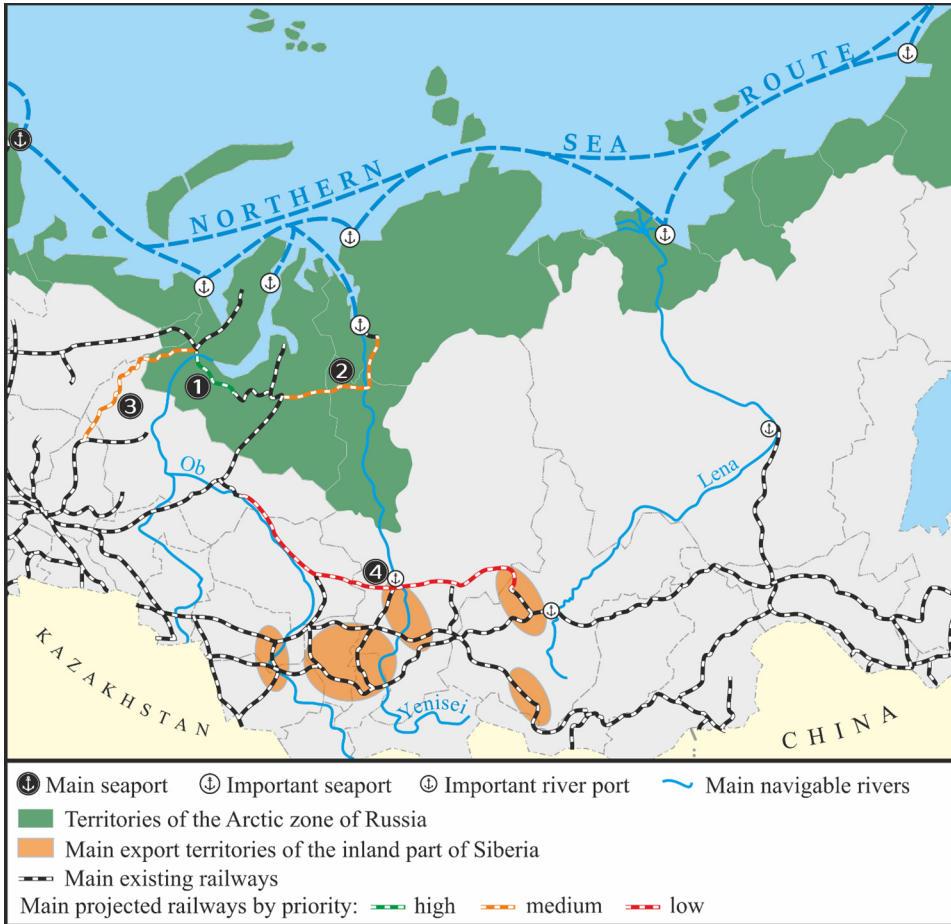
Fig. 3. The Arctic zone of the Russian Federation and the main existing and projected routes of communication with it of the main exporting territories of inland Siberia. The numbers indicate the projected railway lines: 1. Northern latitudinal railway; 2. Northern latitudinal railway – 2; 3. Ural Industrial – Ural Polar; 4. North Siberian Railway
