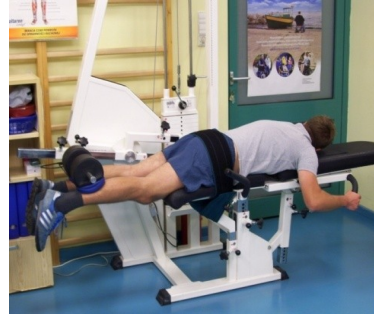
Fig. 10. Static test for flexor in a closed chain (CKC) in the chair tensometric MTD Control.
