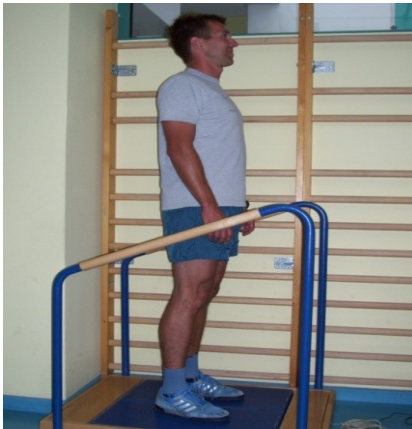
Fig. 6. Static Test Strain gauge platform MTD Control.
