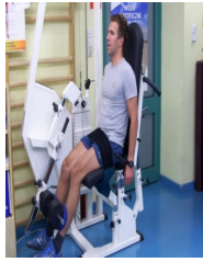
Fig. 2. Static test for extensors 60° in the opened chain (the patient has hands loosely hung) on the armchair tensometric MTD Ctrl.
