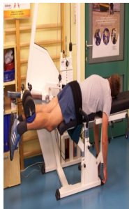
Fig. 4. Static test for flexors in the chain cut open (OKC) on the armchair tensometric MTD Ctrl.
