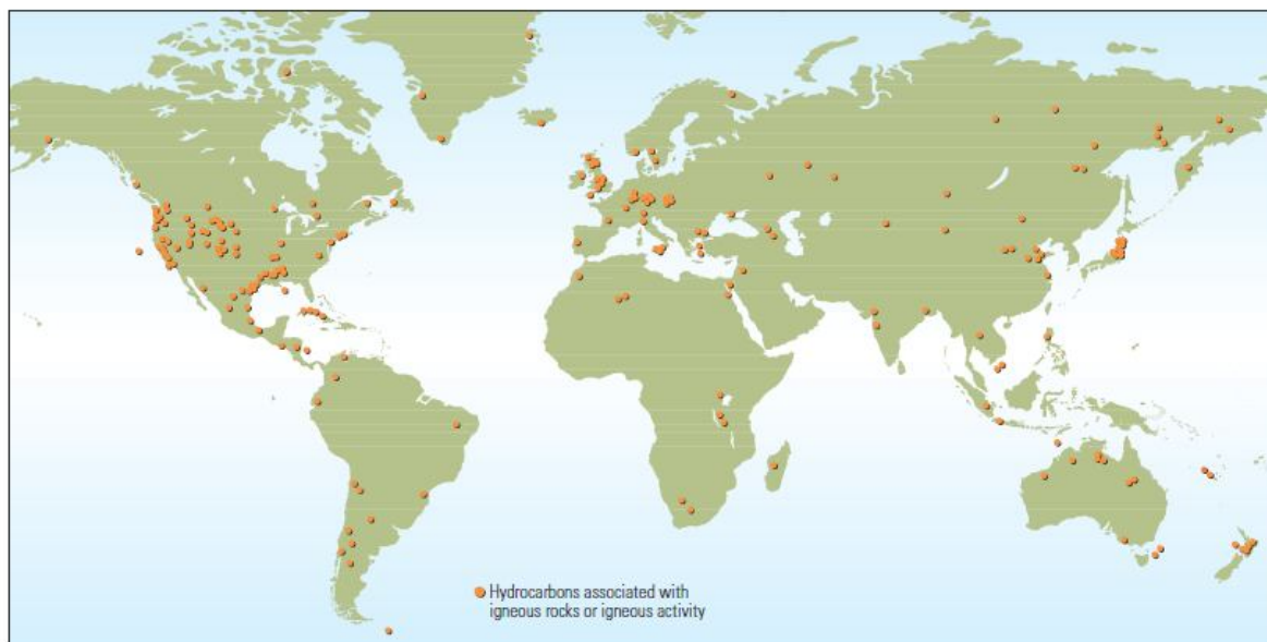
▲ Distribution of hydrocarbon-bearing igneous rocks. Gold dots represent locations of hydrocarbon seeps, shows and reservoirs in igneous rocks. (Adapted from Schutter, reference 36).
