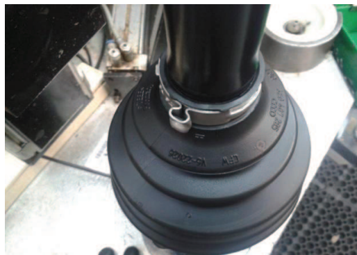
Fig. 2.3. Band installed properly.
