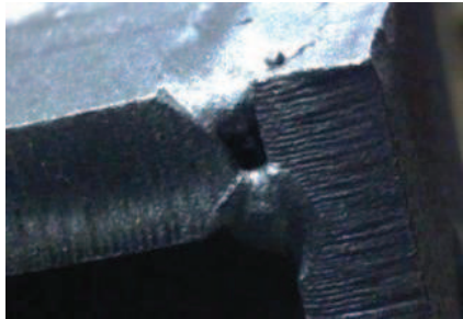
Fig. 7.3. Lack of root fusion.
