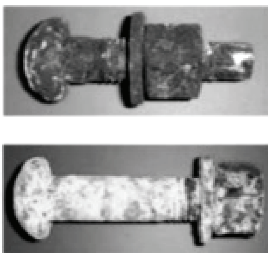
Fig. 11.3. Comparison of methods zinc by using samples after 1500h of salt spray.
