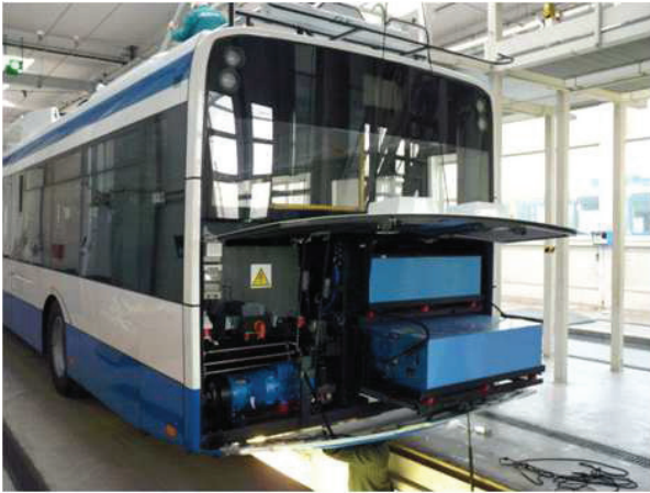
Fig. 2 Traction batteries (right) and DC converter (left)
