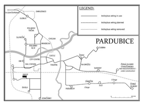
*Fig. 8. The scheme of trolleybus network in Pardubice Author: Maciej Beister*
