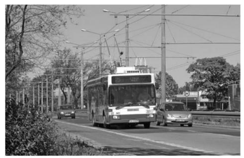
Fig. 4. One of the group of the last five Mercedes O405N converted into trolleybuses in Gdynia, and fitted with a modern asynchronous propulsion system Author: Marcin Połom
