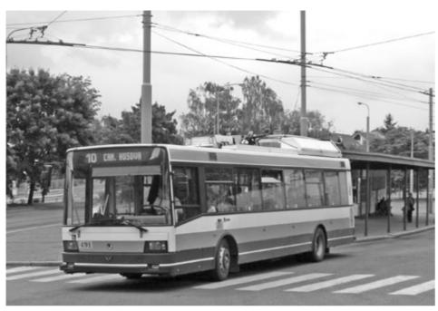
Fig. 4. Low floor trolleybus Skoda 21Tr which is fitted with the diesel aggregate is operated as dual-mode vehicle Author: Mikołaj Bartłomiejczyk
