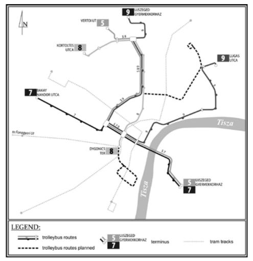
Fig. 1. Scheme of trolleybus routes in Szeged (at 2010) Author: Maciej Beister
