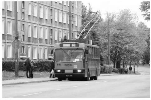
*Fig. 4. Jelcz Pr110E was converted from bus to trolleybus Author: Marcin Połom*
