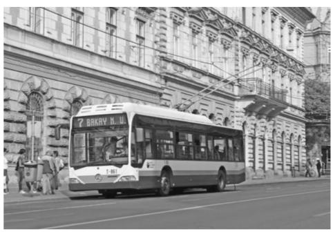
Fig. 4. Converted low floor trolleybus MB Citaro in Szeged Author: Marcin Połom
