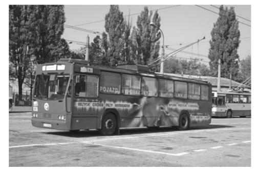
*Fig. 4. Jelcz Pr110 after modernization and replacing electric drive to asynchron Author: Marcin Połom*
