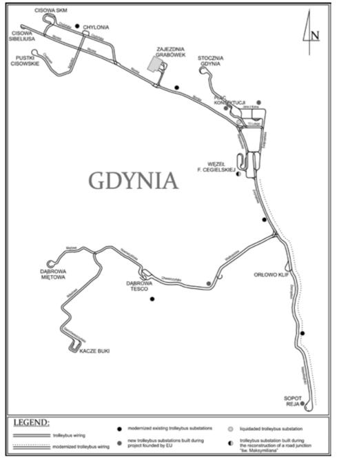
Fig. 9. Scheme of the trolleybus network in Gdynia with the investments realized as a part of the Regional Operational Programme for Pomorskie Voivodeship Author: Marcin Połom, Maciej Beister
