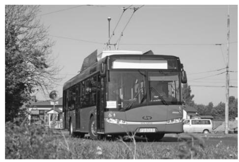
Fig. 3. New type of low floor trolleybus Solaris Trollino with electric drive from polish company Medcom Author: Marcin Połom
