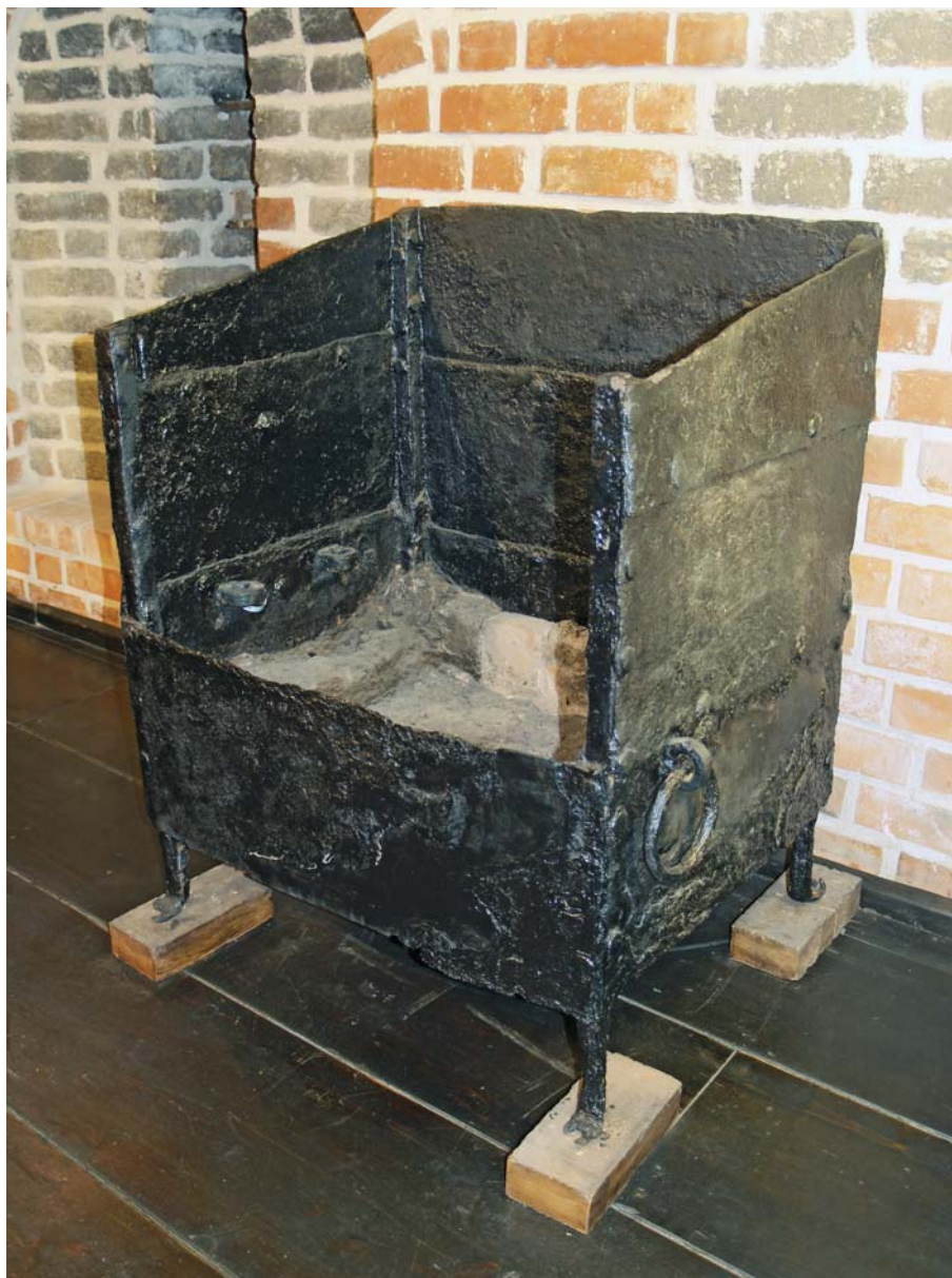
Fig. 3. The stove (firehearth, caboose or camboose) from General Carleton . Possibly manufactured by George Chapman (photo by B. Galus).
