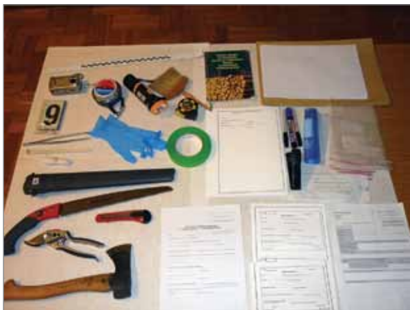
Fig. 3. Handle set “IBL DNA -1” for collection of wood material for DNA analysis
