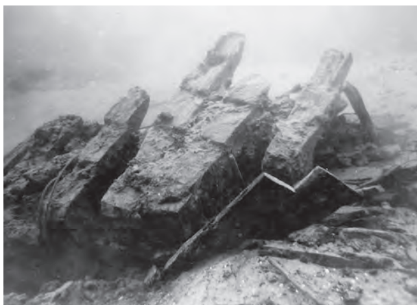
Fig. 27. Stern floor timbers at the bottom of the Gulf of Gdańsk prior to salvage in 1976 (photo by L. Nowicz).
