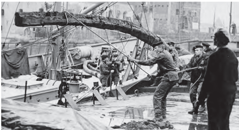
Fig. 26. The keel is transferred to a barge from the deck of a Polish Navy warship using her loading equipment (photo by L. Nowicz).
