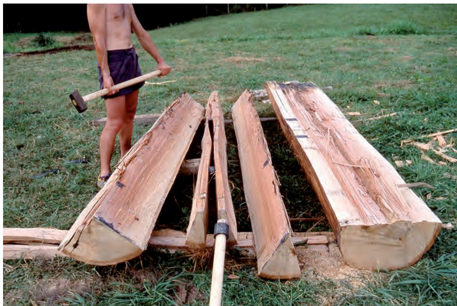
Fig. 12. Reconstruction of oak plank production, after Jean-Albert Glatigny.
