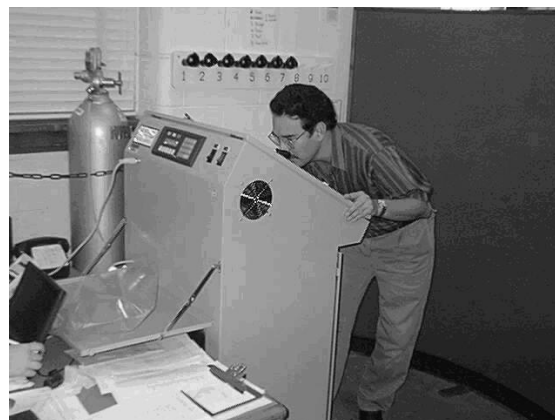
Rys. 2-2 Pomiary olfaktometryczne olfaktometrem AC'SCENT International Olfactometer firmy St. Croix Sensory (Dr. Albert J. Heber, Purdue University, West Lafayette, IN, USA) Fig. 2-2 Olfactometric measurement AC'SCENT International Olfactometer manufactured by St. Croix Sensory (Dr. Albert J. Heber, Purdue University, West Lafayette, IN, USA)
