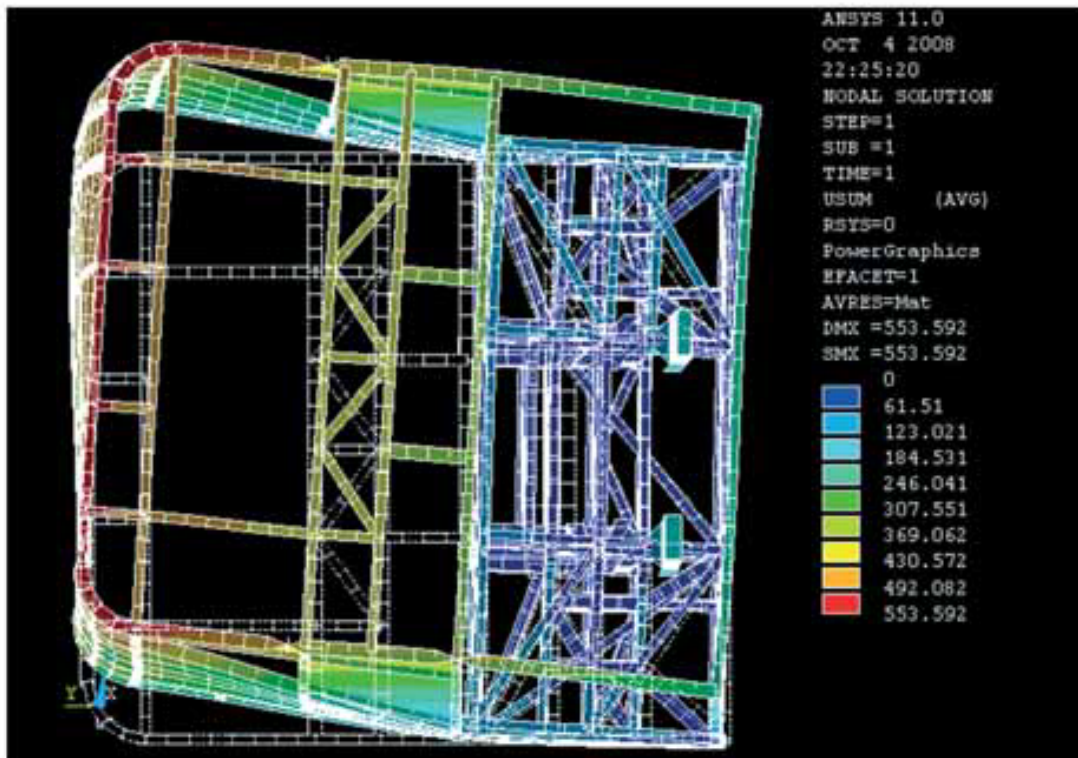
Fig. 9. A model with stiffened rear wall, without roof reinforcements. Contour lines representing the resultant "XYZ" displacements of all the bus body members, viewed from the rear, with reference to the non deformed model
