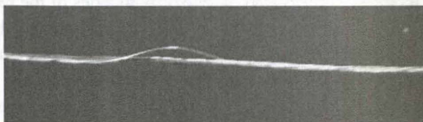
Fig. 12.3. “Loose single wire” discrepancy, illustrated using copper wire.
