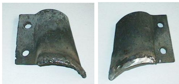
Fig. 8.7. Hard-faced and sharpen blade of the trenching machine.
