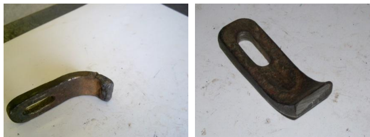
Fig. 5. The hard-faced and sharpen blade for vegetation overgrowth.
