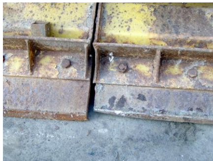
Fig. 8.8. The worn (left) and repaired (right) snow-plough blade.
