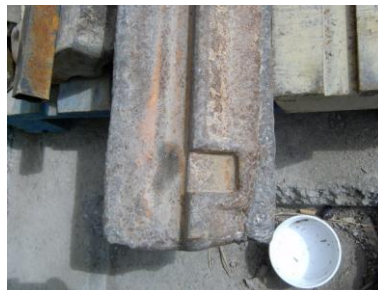
Fig. 8.4. The rock crusher's impact beam.
