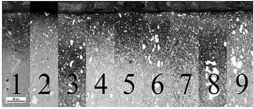
Fig. 9. Structure of the nitrided layers after different activations on X155CrVMo12 steel. Temperature – 813 K, time – 3 h. Optical microscopy images, samples were etched by 4% \text{HNO}_3 /ethanol.
