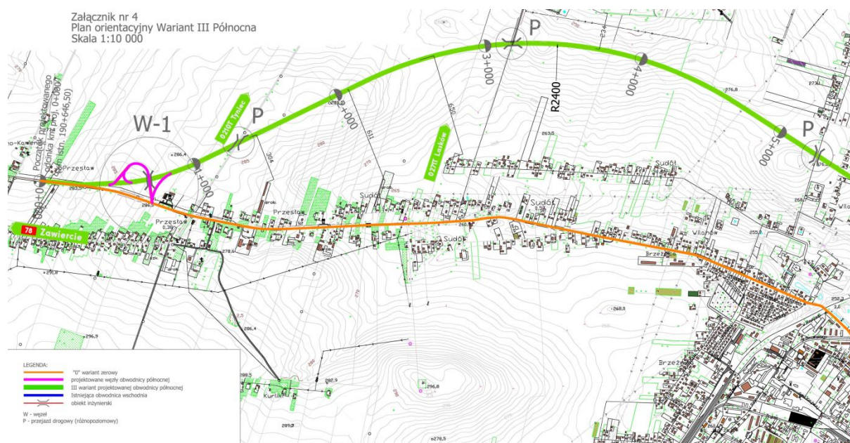
Fig. 4. Topographic map with the proposed bypass being part of national road (fragment). Source: Own elaboration based on the documentation available at https://www.gddkia.gov.pl
