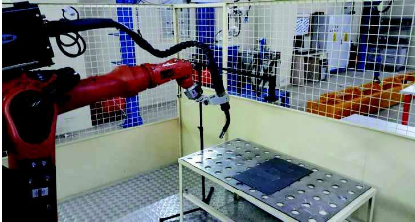
Fig. 1. Experiment system with industrial welding robot and camera.
