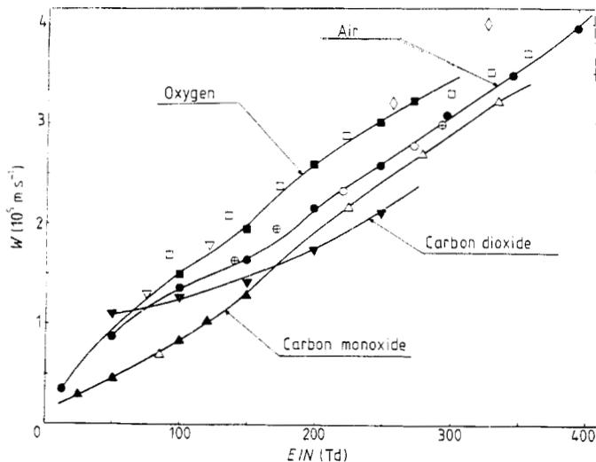
**Figure 4.** Drift velocities in oxygen, carbon monoxide, carbon dioxide and air at moderate  $E/N$ . Oxygen:  $\square$  (Frommhold 1964);  $\nabla$  (Naidu and Prasad 1970);  $\diamond$  (Schlumbohm 1965);  $\blacksquare$  (present results). Carbon monoxide:  $\triangle$  (Saelee 1976);  $\blacktriangle$  (present results). Carbon dioxide:  $\blacktriangledown$  (present results). Air:  $\circ$  (Frommhold 1974);  $\oplus$  (Ryžko 1965);  $\bullet$  (present results).
