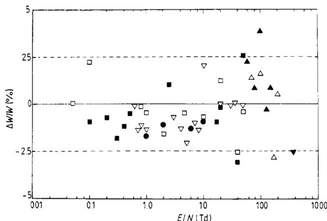
**Figure 2.** Percentage difference between the present results and those of other investigators for hydrogen, nitrogen, and carbon dioxide. Hydrogen: ■ (Lowke 1963); ● (Robertson 1971); ▲ (Blevin and Hasan 1967); ▼ (Saelee 1976). Nitrogen: □ (Lowke 1963); △ (Blevin and Hasan 1967). Carbon dioxide: ▽ (Elford and Haddad 1980).
