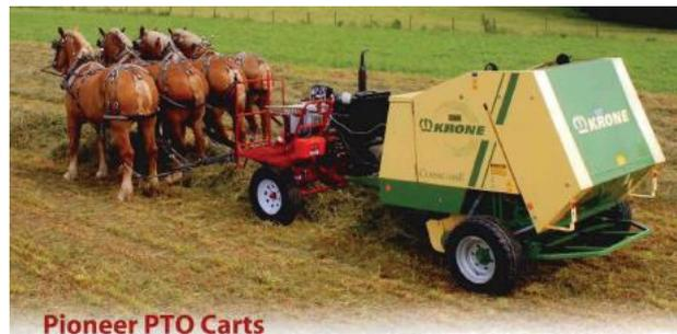
Figure 5. Forecart with engine PTO (Pioneer catalog 2014)
