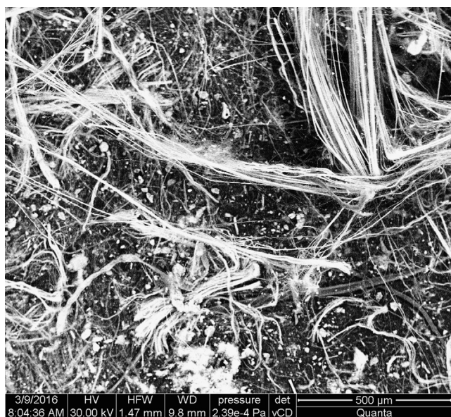
Fig. 2. Microphotograph of asbestos cord sample prior to its digestion; magnification 200×.
