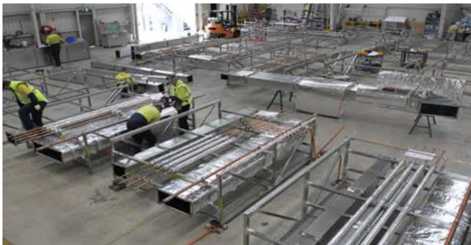
Fig. 1. Prefabricated horizontal distributions of sanitary installations for a hospital facility in Australia
