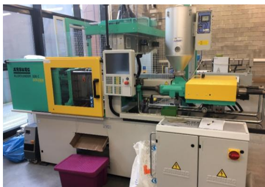
Fig. 1 Injection moulding machine type Arburg Allrounder 320 C
