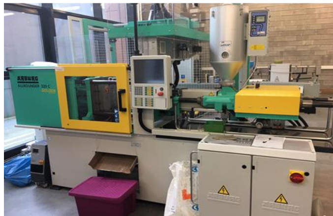
Fig. 2. Injection moulding machine Arburg Allrounder 320 C used for testing
