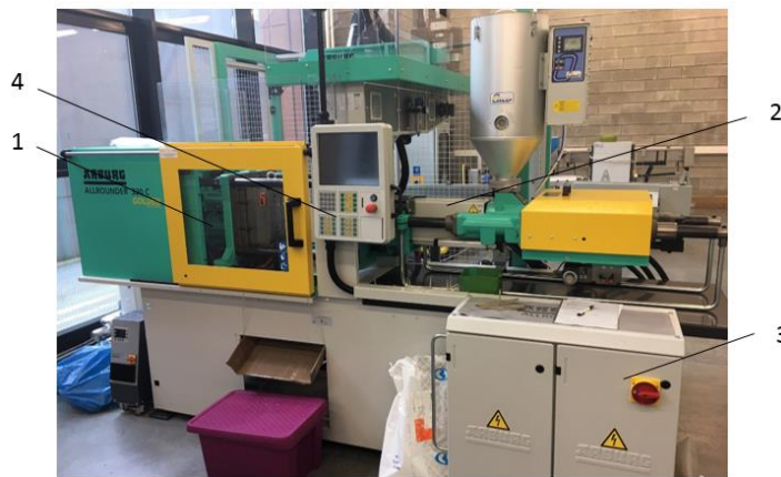
Fig. 3. Injection moulding machine Arburg Allrounder 320 C used for testing 1 – tool system, 2 – plasticizing system, 3 – drive system, 4 – control device
