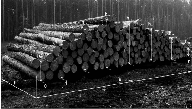
Figure 1. Elements of irregular stack measurement ( h_0-h_n – height, l – stack length, s – stack width)
