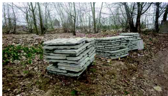
Fig. 2. Storage of concrete elements on wooden pallets
