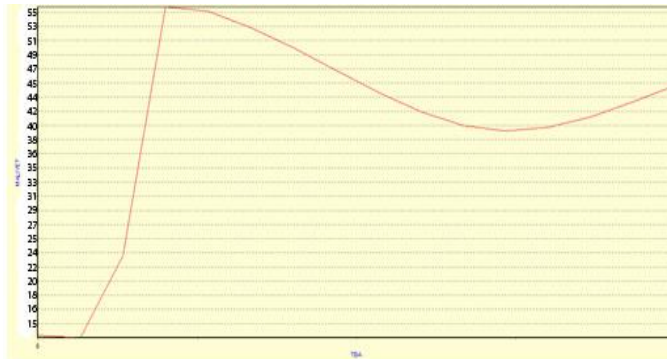
Fig. 16. The relationship between the total balcony area and the cost of the building unit (m 2 )
