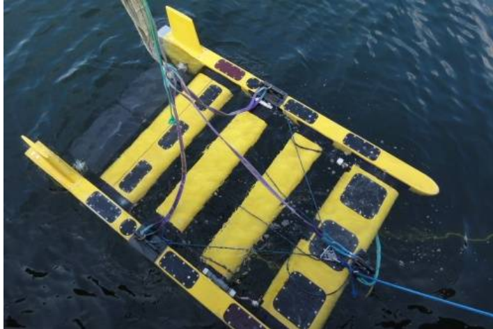
BURMIN with characteristic stabilization fins (towing by the USV) as a part of MCM system
