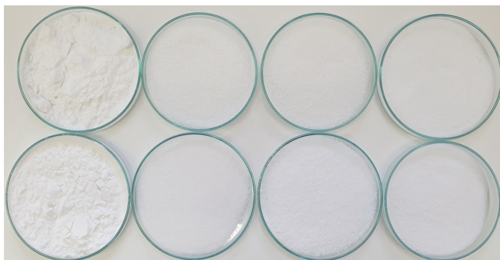
Figure 5. Photograph of raw material and obtained aerogel samples (from left: native starch, aerogel, E 1422 aerogel, and E1450 aerogel; from top: native and waxy variety, respectively).
