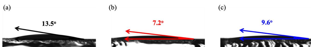
Figure S6. Water contact angle measurements on (a) ZnO; (b) AZO-1 and (c) AZO-2 ETLs.
