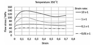
Figure 4 Flow stress curves of ZK60 cast alloy at a temperature of 350 °C
