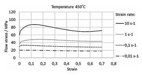
Figure 6 Flow stress curves of ZK60 cast alloy at a temperature of 450 ℃
