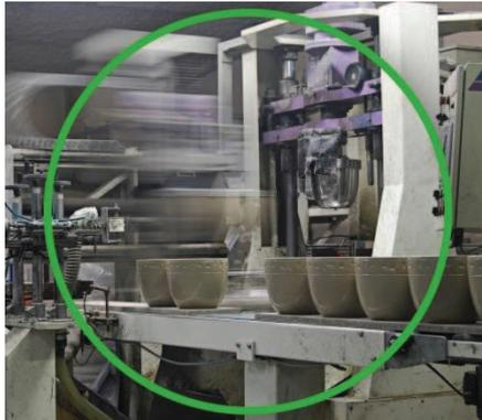
**Fig. 8.1. Hydraulic press – potsherd moulding**
