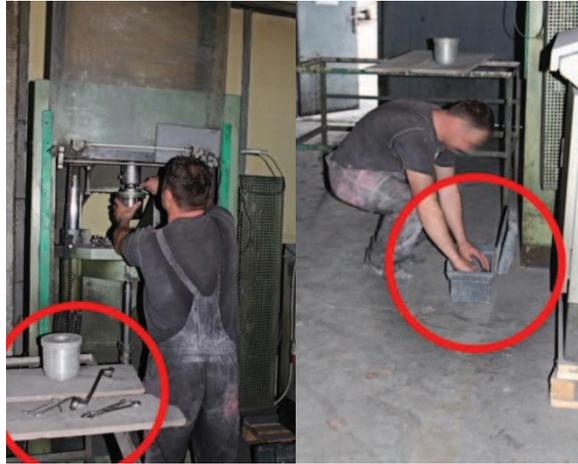
**Fig. 8.2.a) Hydraulic press – changing of the mould before implementation of changes, b) hydraulic press – looking for tools before implementation of changes**
