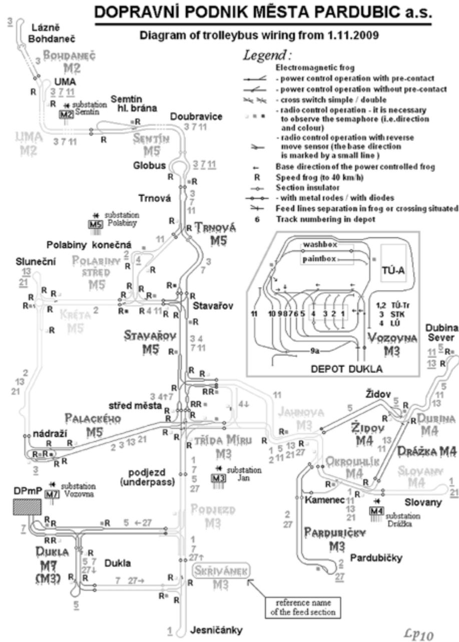
Fig. 10. The scheme of trolleybus network in Pardubice
