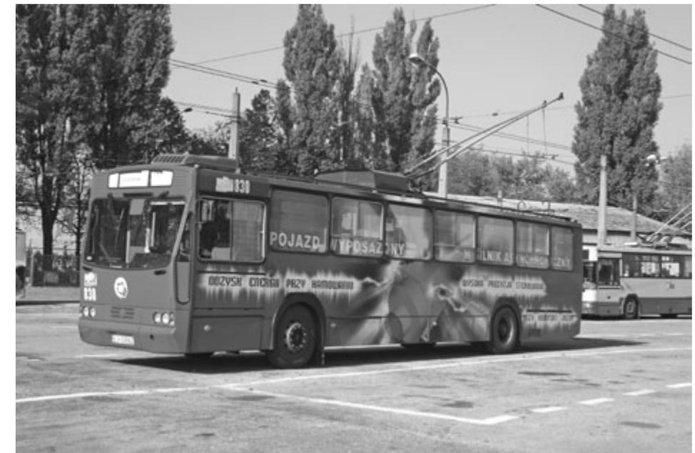
Fig. 4. Jelcz Pr110 after modernization and replacing electric drive to asynchron
