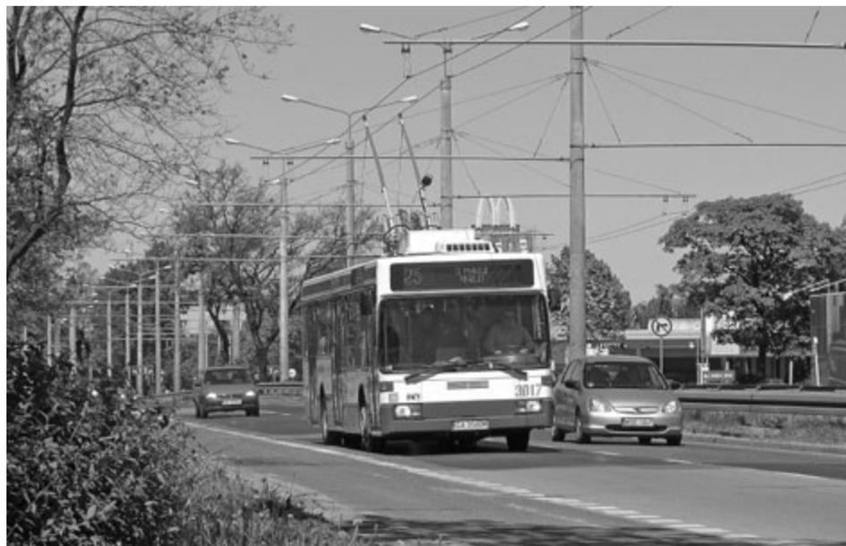
Fig. 4. One of the group of the last five Mercedes O405N converted into trolleybuses in Gdynia, and fitted with a modern asynchronous propulsion system
