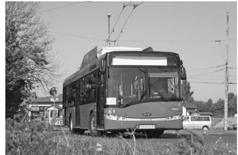
Fig. 3. New type of low floor trolleybus Solaris Trollino with electric drive from polish company Medcom
