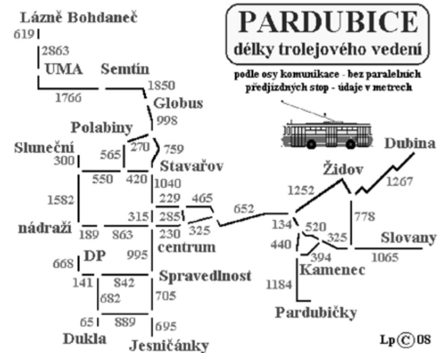
Fig. 9. Lengths of the particular sections of the trolleybus system
