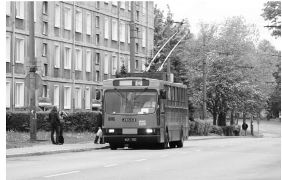
Fig. 4. Jelcz Pr110E was converted from bus to trolleybus
