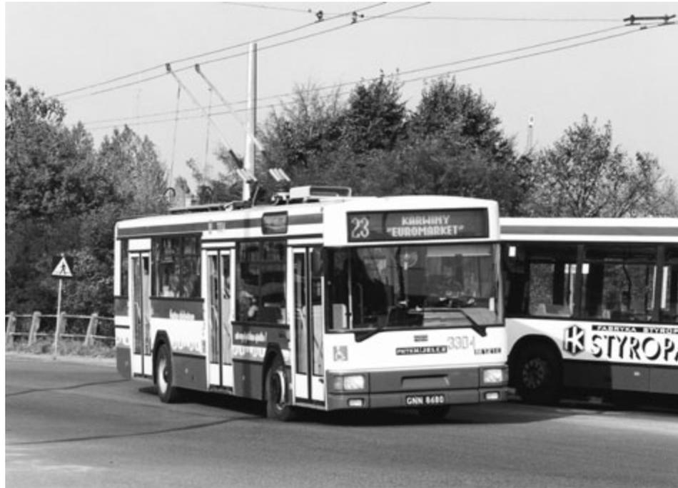
*Fig. 1. Low entrance trolleybus PNTKM/Jelcz M121MT
