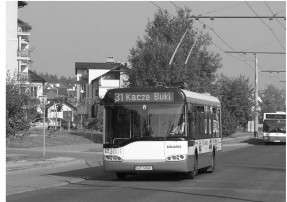
*Fig. 2. Low floor Solaris Trollino 12T trolleybus constructed by PNTKM in Gdynia
