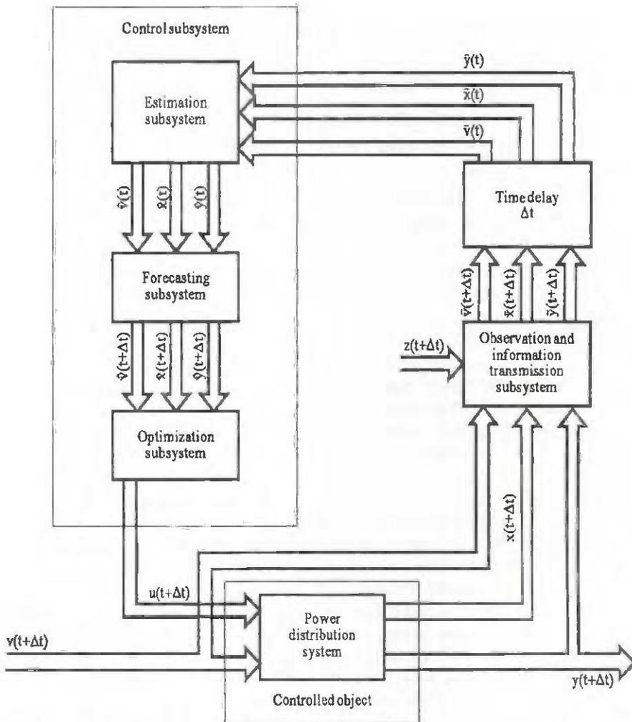
Fig. 2.1. The diagram of the information structure of the real time control system of the operation of electrical power distribution systems.
